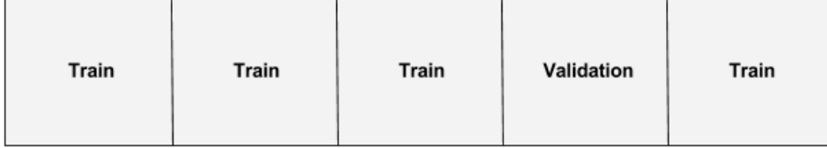
Figure 2: 5-fold cross-validation. The n observations are divided into five subsets. A model is fitted to the validation subset by using the four training subsets. This is done for all five subsets.
