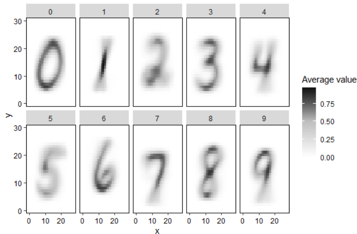
Figure 17: The centroids of each digit of the MNIST data where each pixel is the average pixel value of the particular digit. (X, Y) represent the frame of each image and consist of 28 pixels each. The legend shows the grey-scale of every average pixel value.
