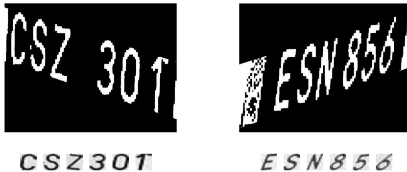
Figure 11: License plate & detected characters after removing above and below the characters.
