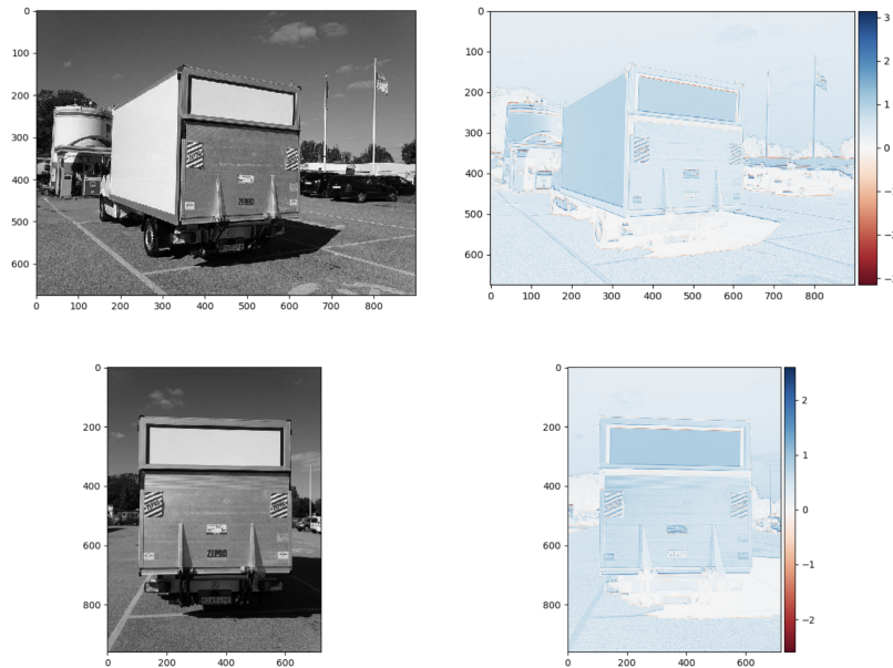
Figure 3: Left: original image, right: Sobel filter.
