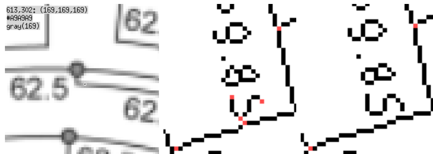
Figure 6.2: Graph 4, where left image had spots missed by threshold 130, middle shows intersection at threshold 180, right shows result using threshold 175. (Frygelius et al. 2010). Republished with permission of Copyright ©John Wiley Sons – Books 2010, from Evolution and human tissue expression of the Cres/Testatin subgroup genes, a reproductive tissue specific subgroup of the type 2 cystatins , Frygelius et al., 12, 3, 2010; permission conveyed through Copyright Clearance Center, Inc.
