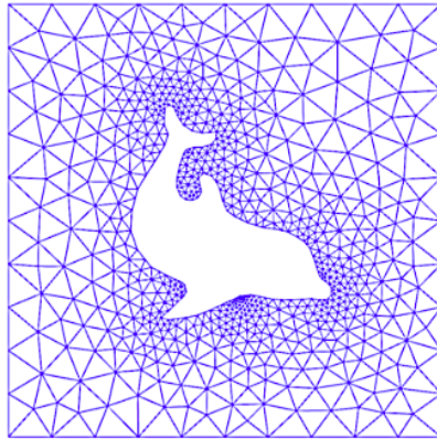
Figure 2.2: An unstructured mesh where the boundary is in the shape of a dolphin. The figure is taken from [11].
