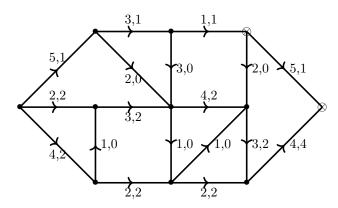
We find a cut with capacity 5 too. One such cut is  $(P, P^c)$  where  $P^c$  contains exactly the sink z and the unique adjacent vertex v such that (v, z) has capacity 5. The two vertices are marked in the graphic. By the max-flow-min-cut theorem, this already shows that the found flow is maximal and the indicated cut is minimal.
