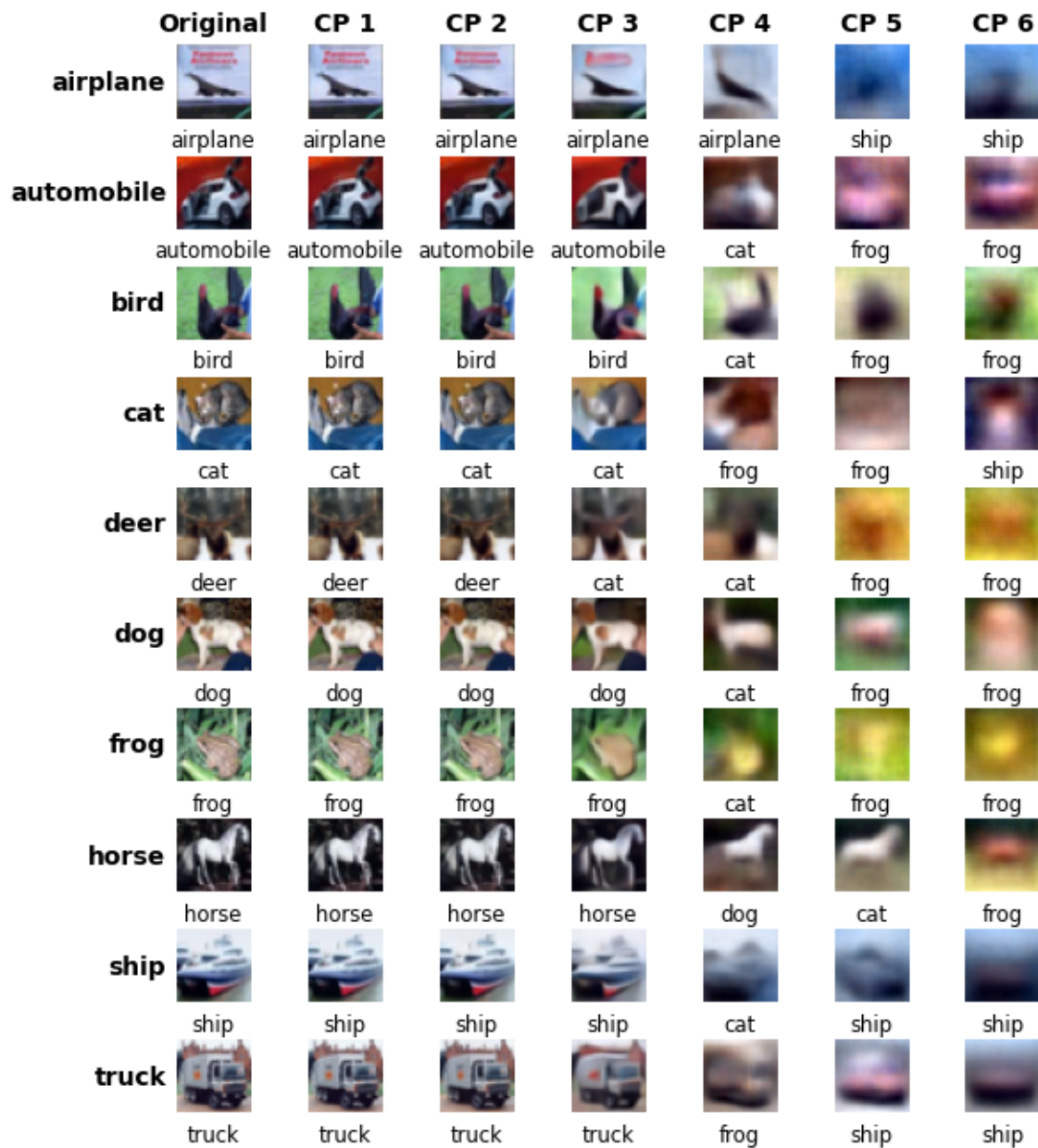
Figure 14: Examples of decoded images from each checkpoint, along with the corresponding original image which was correctly classified by ResNet-18. Each row is labelled with the class of the original image. Underneath each image, the prediction of ResNet-18 is displayed.
