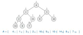
To transform A into a max-heap, we may simply apply Max-Heapify bottom-up to each i violating the max-heap property.
