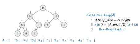
To transform A into a max-heap, we may simply apply Max-Heapify bottom-up to each i violating the max-heap property.
