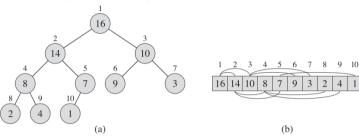
Number within the circle at each node in the tree is the value stored at that node. The number above a node is the corresponding index in the array. Above and below the array are lines showing parent-child relationships; parents are always to the left of their children.
