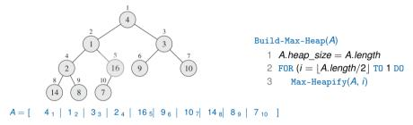
To transform A into a max-heap, we may simply apply Max-Heapify bottom-up to each i violating the max-heap property.
