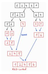
The key idea of the "merging-operation" is the merging of two sorted sequences which is done by calling an auxiliary procedure
