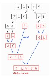
The key idea of the "merging-operation" is the merging of two sorted sequences which is done by calling an auxiliary procedure
