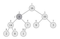
Max-Heapify lets the value at A[i] "float down" in the max-heap so that the subtree rooted at index i obeys the max-heap property.
