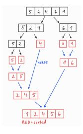
The key idea of the "merging-operation" is the merging of two sorted sequences which is done by calling an auxiliary procedure
