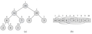
Number within the circle at each node in the tree is the value stored at that node. The number above a node is the corresponding index in the array. Above and below the array are lines showing parent-child relationships; parents are always to the left of their children.
