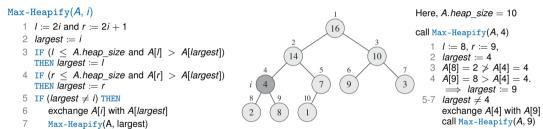
Max-Heapify lets the value at A[i] "float down" in the max-heap so that the subtree rooted at index i obeys the max-heap property.
