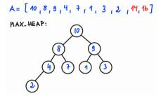
Aim: Order elements of a given array A = A[1..n] such that  $A[1] \le A[2] \le \cdots \le A[n]$ . Heapsort Alq. Idea:
