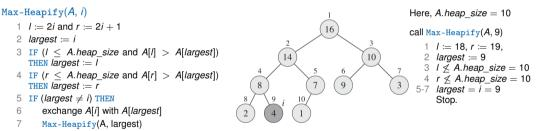
Since we always exchanged with largest child-value, the final tree T(i) is a max-heap.
