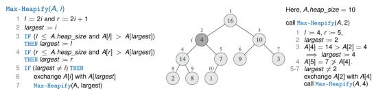
Max-Heapify lets the value at A[i] "float down" in the max-heap so that the subtree rooted at index i obeys the max-heap property.
