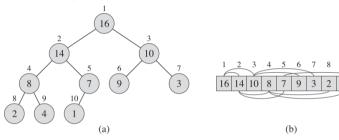
Number within the circle at each node in the tree is the value stored at that node. The number above a node is the corresponding index in the array. Above and below the array are lines showing parent-child relationships; parents are always to the left of their children.
