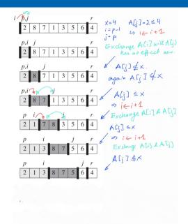
The key to Quicksort is the Partition procedure, which rearranges the subarray A[p..r] in place.
