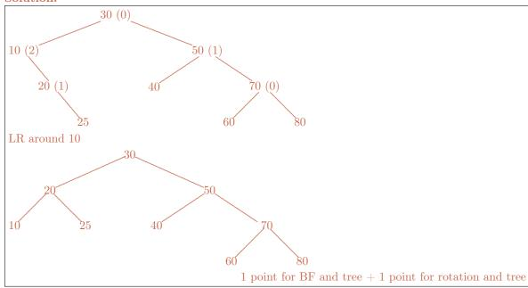
(b) Delete 30 from the tree T and draw the resulting tree "T-30" including the balance factors next to each inner vertex. If "T-30" is not an AVL tree, rebalance it. Specify the rotation(s) for rebalancing and draw the resulting tree after rebalancing it.
